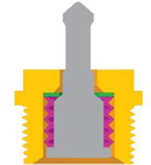
[Cross-Sectional View of the Defendant's Product "Stud Socket Ass'y"]
