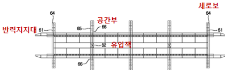
[Drawing 4] Plane View that Illustrates the Installation of Double Girders on Workbench Illustrated in Drawing 3
